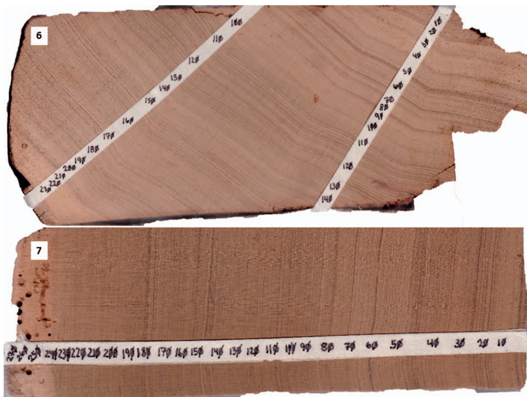
Figures 6–7.—Tulip poplar tree-ring samples. (6) Sample TRC01A (1561–1803). This tulip poplar sample was obtained from the attic of the Territorial Capitol (Vincennes) during renovation. Since dating the ring adjacent to the bark was possible for this sample, we were able to determine when the tree was cut and used in construction (1803). Numbers on the sample indicate individual decades of growth. (7) Sample KEL69A, a wall stud obtained from the Kellems House. The tree rings in the sample date from 1564 to 1836. The growth in this sample is extremely compact, and mean ring width is a mere 0.56 mm ( \pm 0.24 SD).
