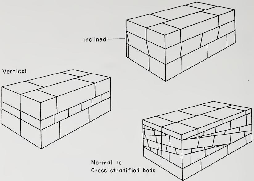
FIGURE 1. Block diagram showing three basic types of jointing.
