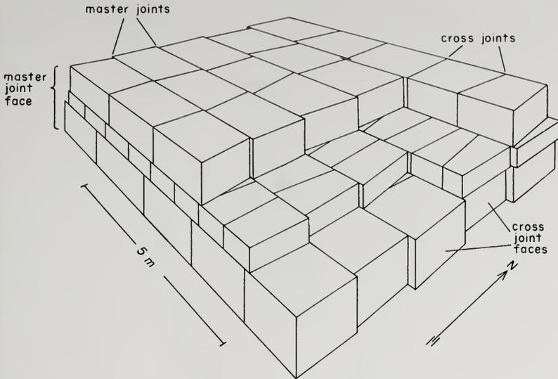
FIGURE 2. Block diagram showing idealized sets of master and cross joints in three beds of rock.
