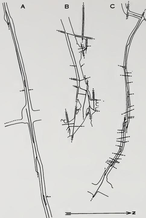
FIGURE 3. Maps showing the relationship of joints (heavy lines) to portions of cavern passages in various stratigraphic units.
