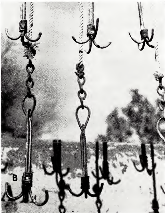
FIGURE 2. A. Johuboa t with crowfoot bar on stanchions. B. Detailed view of crowfoot hooks.
