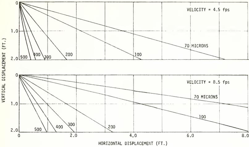
FIGURE 3. THEORETICAL TRAJECTORIES OF SPHERICAL PARTICLES IN A HORIZONTAL AIR STREAM
