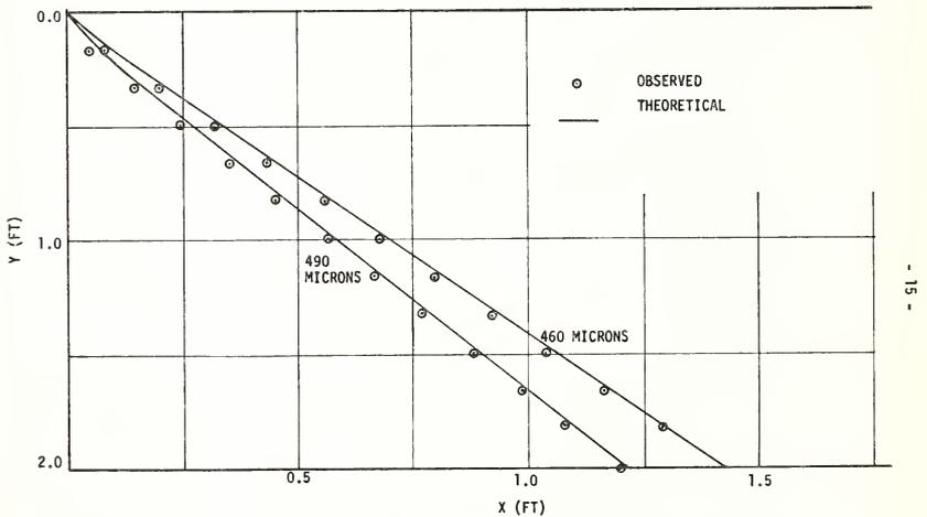
FIGURE 6. THEORETICAL AND OBSERVED TRAJECTORIES FOR A VELOCITY OF 10 FT./SEC.
