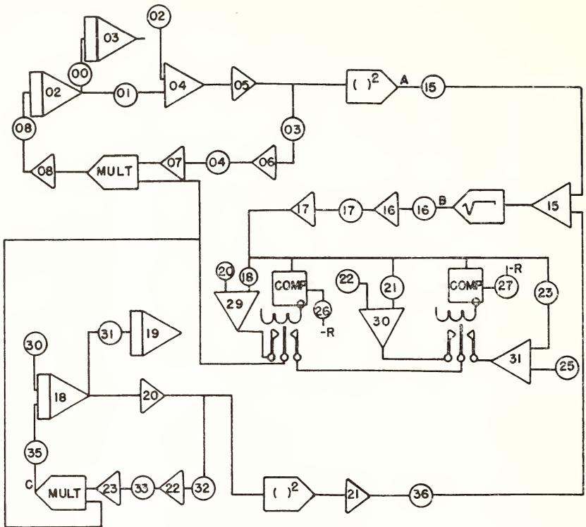
FIGURE 2. A SCHEMATIC DIAGRAM OF THE ANALOG COMPUTER SOLUTION OF THE EQUATIONS OF MOTION FOR A SPHERICAL PARTICLE IN AN AIR STREAM.
