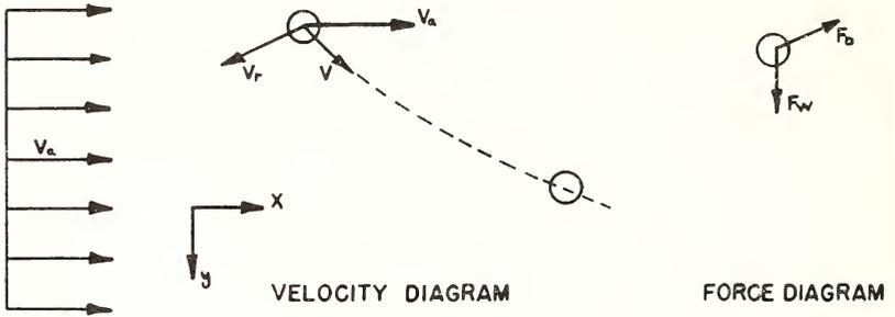
Figure 1. Velocity and Force Diagrams for a Particle in a Horizontal Air Stream.
