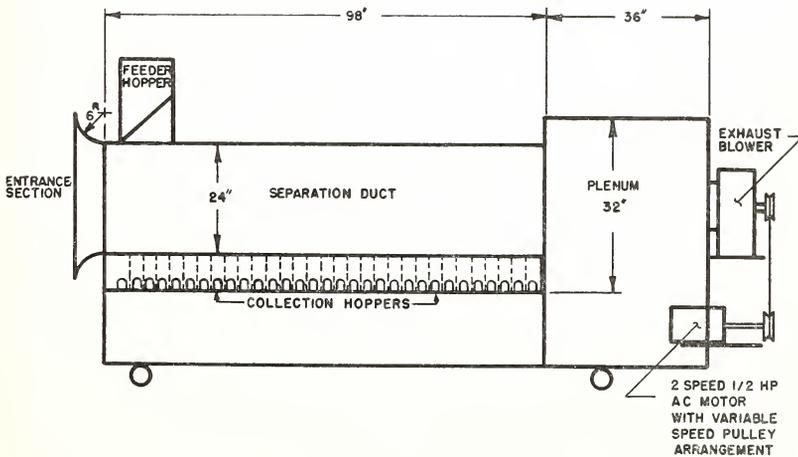
FIGURE 4. A SCHEMATIC DRAWING OF THE SEPARATOR
