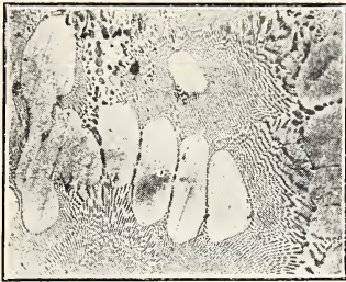
Fig. 32—Cadmium-tin eutectoid with excess of tin. \times 100 .
