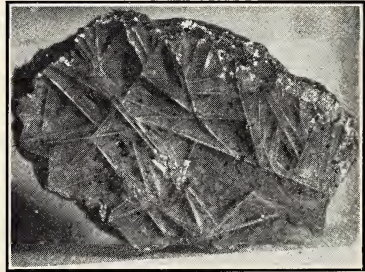
Fig. 2—Surface of ferrosilicon. Skeleton of skin first frozen. x1/4.
