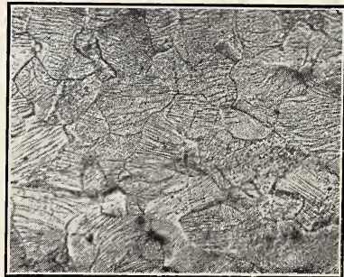
Fig. 14—Slip bands in strained ingot iron. x130.
