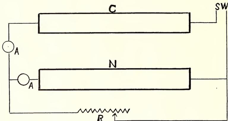
Fig. 2—Diagram of apparatus used in insulation tests.
