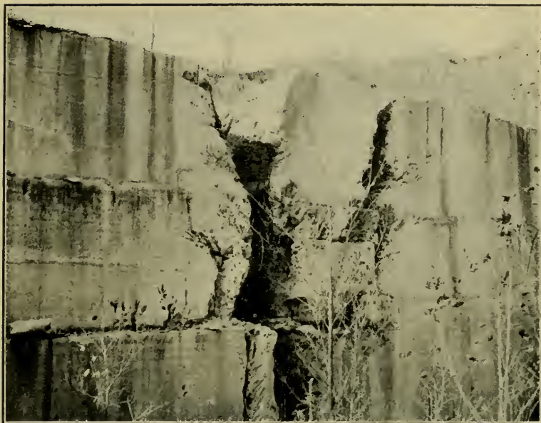
No. 11. Old Quarry one mile west of Stinesville, showing joint enlarged by solution. Salem limestone.
