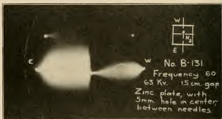
Fig. 5. Discharge in nitrogen passing through hole in zinc plate. Note unidirectional effect.
